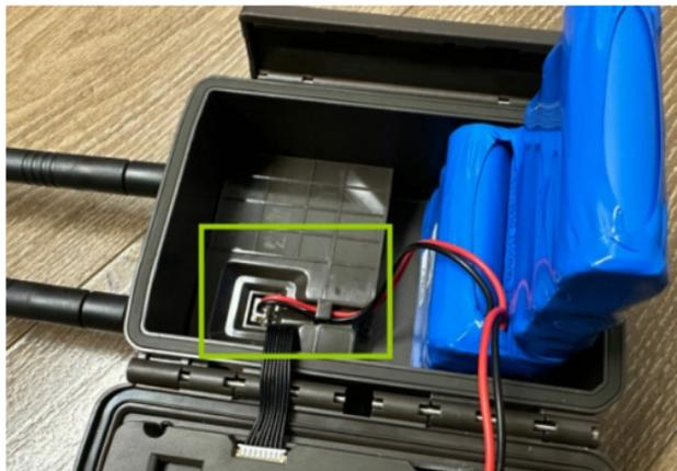
Step3: Insert the other power port into the main board's power interface.
