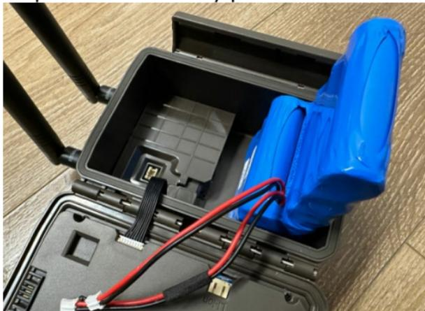
Step2: Insert the power port into the module's power interface. Then press the wire into the take-up slot.
